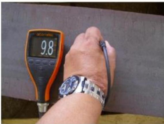
Mill scale with 80% magnetite ( $\text{FeO} \cdot \text{Fe}_2\text{O}_3$ ), thickness is 9.8 microns.
